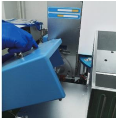
Figure-22 Opening the protective cover
