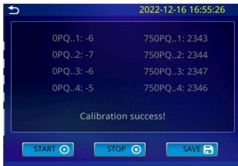
Figure-13 Shows the signal value of the standard sample
