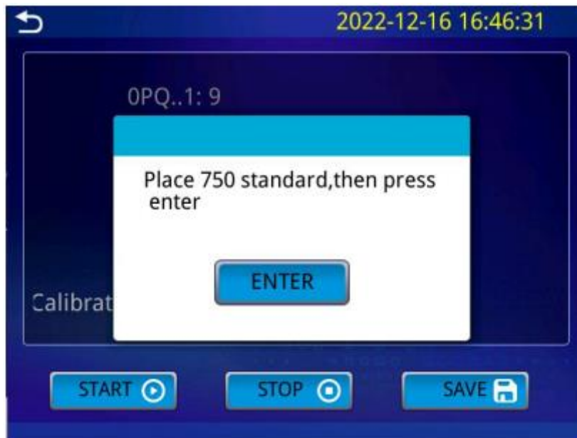
Figure-12 750 standard oil sample calibration interface
